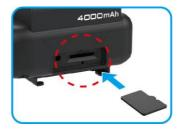
The slot cover must be tightly sealed to prevent moisture from entering, causing the lens to fog. Insert the left edge of the slot cover, and then press the right edge of the slot cover to create a good seal. See below.
