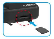
The slot cover must be tightly sealed to prevent moisture from entering, causing the lens to fog. Insert the left edge of the slot cover, and then press the right edge of the slot cover to create a good seal. Same as USB cover. See below.
