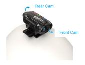
3 Make sure your phone is connected with MUFU\_V40T\_xxxx via Wi-Fi, and open the MUFU Video app to check preview image. Move right or left, forward or backward the mount to obtain the best recording image angle.
